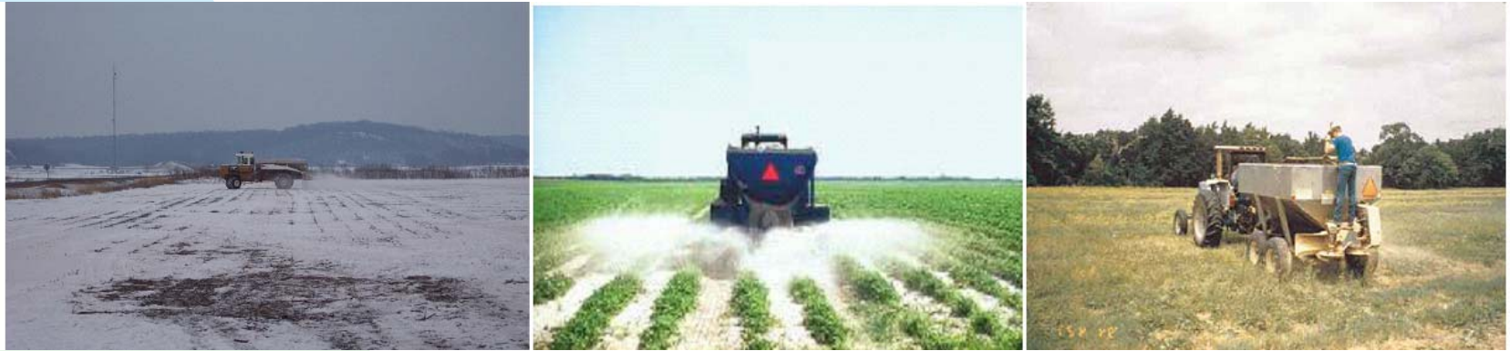
Figure 4-1. FGD gypsum can be applied directly to the soil surface using conventional dry material spreaders (Source: National Research and Demonstration Network of FGD products in Agriculture).
